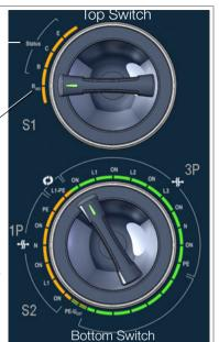
Orange switch positions: testing at single-phase, mode 2/3 cables Green switch positions: testing at 3-phase, mode 2/3 cables
